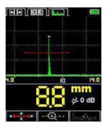
For measurings with displaying signals as A-Scan. This mode makes it possible to rule out inaccuracy of measurements caused by duplicated readings. There are four possible ways to conduct measuring:
